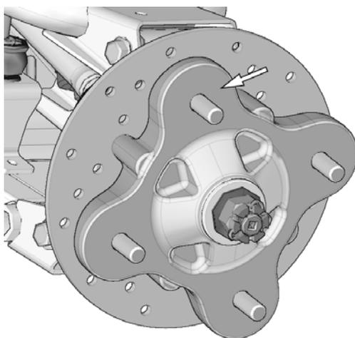
3. If applicable, remove CV joint protectors.
