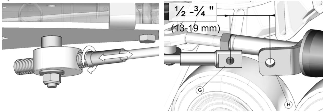
14. Reverse steering wheel a little to be able to bolt support plate and cable together. Tighten provided bolt (**i**) to 35 N•m [24 lb•ft]. See Figure 24. Repeat steps for right side.
