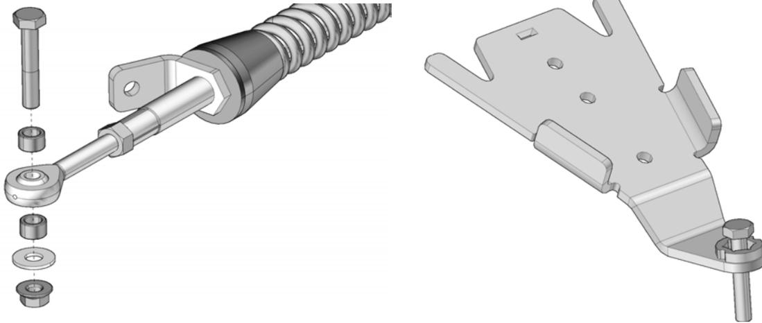
5. Position the bottom part of the anchor bracket (2) underneath the lower suspension arm. Position the top part (3) over the suspension arm so the tenon slips in the mortise cut in the bottom part. Insert the M10x55 mm bolts (4) through the bottom and secure the two parts together with the nuts (5) provided. Tighten assembly to 50 N•m [37 lb•ft] of torque. Refer to Figure 15.
