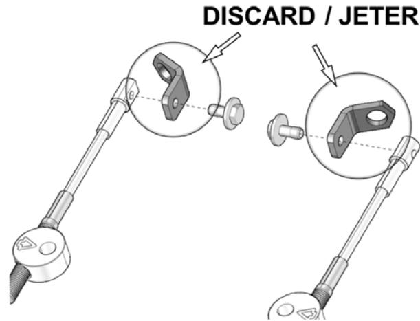
8. Discard the M10x60mm bolts (20) from steering limiter assembly kit. See Figure 21.
