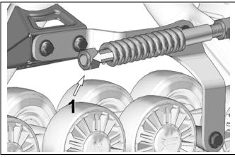
• Loosen the nut (1) compressing the spring of the stabilizing rod. See Figure 8.
