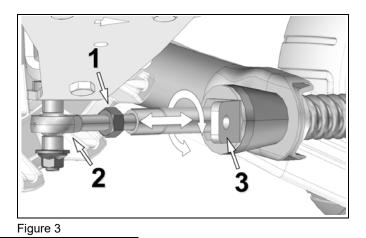
When angle of attack is correctly set, tighten the jam nut (1) back against the stabilizing arm to 40 N•m [30lb•ft] of torque. See Figure 4.
