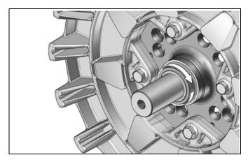
NOTE: Replace Speed Sleeve immediately if defective.
