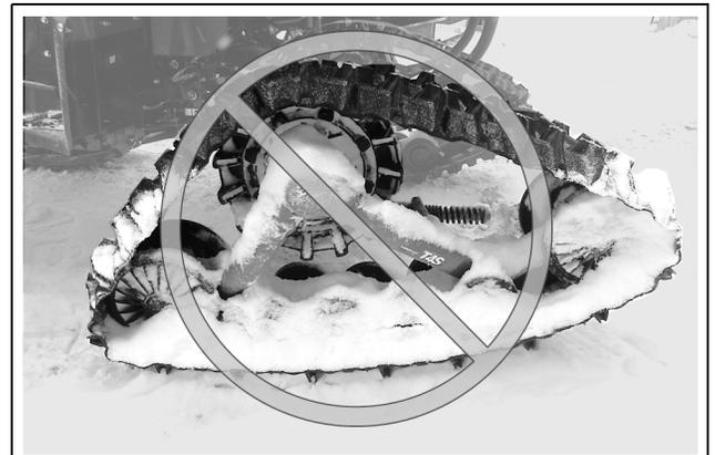
**CAUTION:** Track systems installed on an ATV project more snow, dirt, water, or mud than tires. The owner/driver is responsible for adapting engine and CVT air intakes to minimize the risks of breakdowns and/or damage to mechanical components.
