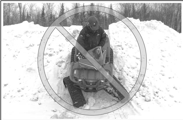
**CAUTION:** During a steep descent, it is advisable to keep the handlebars straight and to begin turning when the ATV is on flat ground, thus avoiding subjecting the vehicle components and the System to any high stress.
