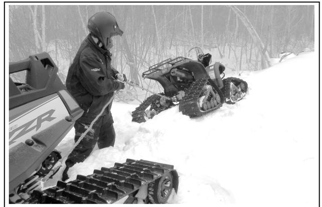
**CAUTION:** Tow the vehicle back in the direction of the tracks left before getting stuck.
