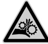
**Moving Parts** - Hands or fingers caught between moving parts of the equipment present a danger to life or limb. Turn motor off before servicing the Track System.
