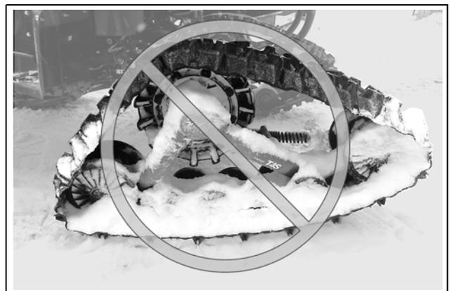
**CAUTION:** Track systems installed on an ATV or SxS project more snow, dirt, water, or mud than tires. The owner/driver is responsible for adapting engine and CVT air intakes to minimize the risks of breakdowns and/or damage to mechanical components.
