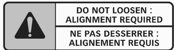
**TENSIONER BOLT WARNING** - If track tension adjustment is required, do not loosen the tensioner assembly bolt under any circumstance. The bolt is used to assemble and align the tensioner with the frame. Tensioner re-alignment is necessary if this bolt is loosened.
