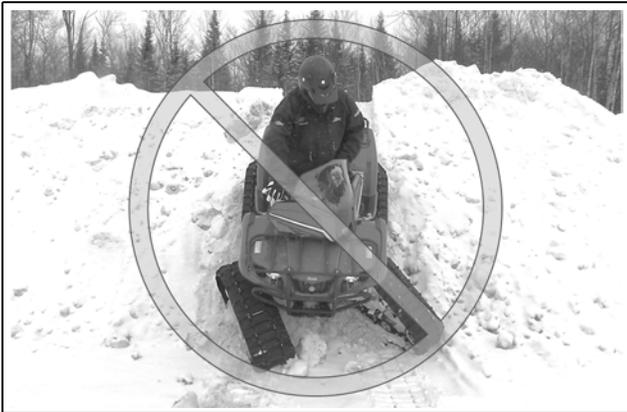
**CAUTION:** During a steep descent, it is advisable to keep the handlebars straight and to begin turning when the vehicle is on flat ground, thus avoiding subjecting the vehicle components and the System to any high stress.
